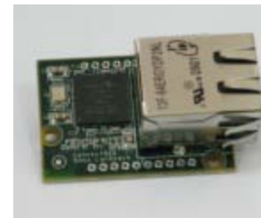
Nano LANReach 3-24Mbps Ethernet module with server.
